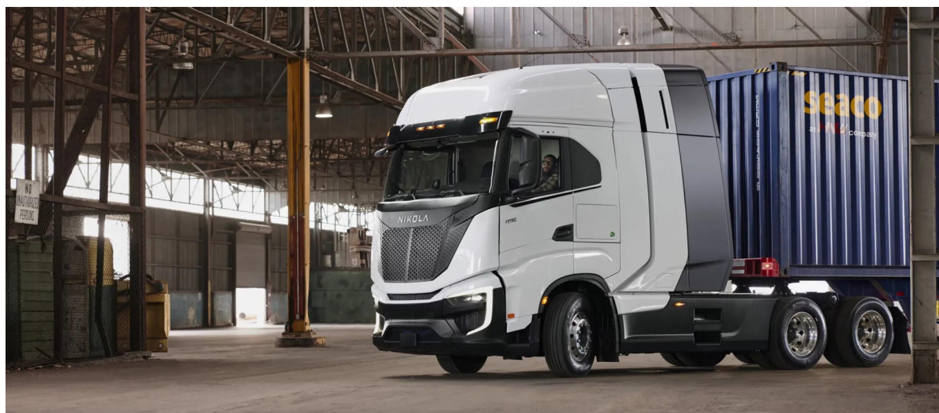
The Nikola Tre hydrogen fuel cell truck relies on type 4 hydrogen cylinders from Hexagon Purus
