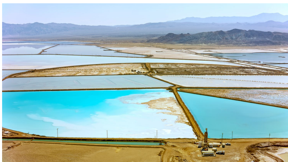
Figure 1. Lithium Brine Evaporation Ponds at Silver Peak, Nevada
